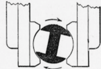
FIG. 4. POSITION OF MAGNETO ARMATURE WHEN CONTACTS SHOULD OPEN
