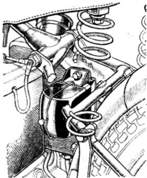
The position of the Lucas automatic voltage control on the new A.J.S.s.
