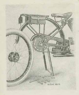
A.J.S. Quick-Detachable Wheel, as fitted to Models E3 and E4.
