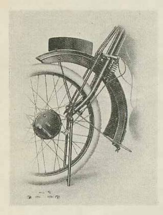
Removing Front Wheel—Disconnect cable yoke end from brake operating lever, remove anchor plate bolt from fork end, and after slackening off spindle nuts the wheel will then fall out of slots in fork ends.
