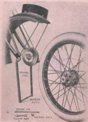
Showing Front Wheel detached and its interchangeability with Rear Wheel.
