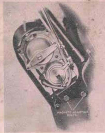
Lucas "Magdyno" in position, showing adjustment.
